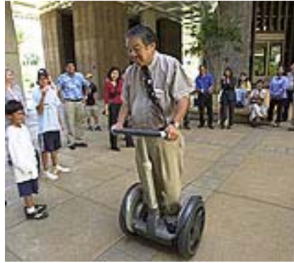
Figure 1. Segway 20km/h gyroscopically balanced powered mobility platform
